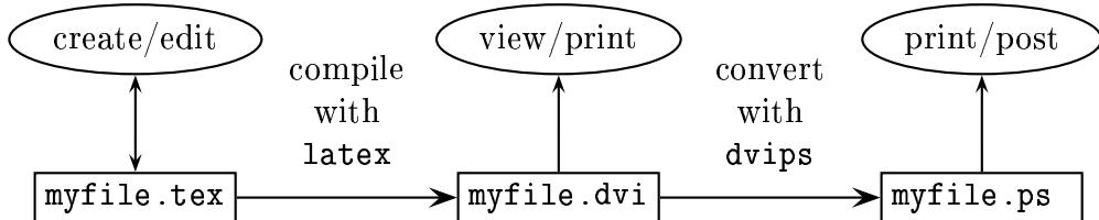
Figure 3: Command Sequence from Source to Postscript
